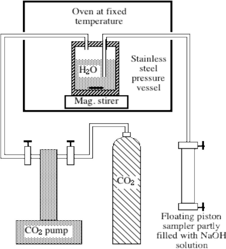
Figure 3 Simplified schematic of column experiment layout.
