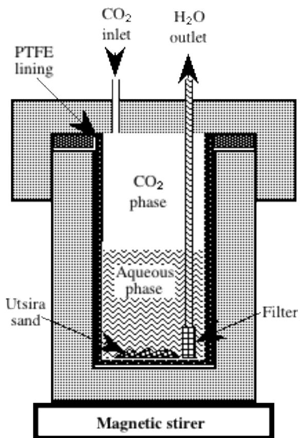
Figure 2 Schematic diagram showing the sampling of a batch reactor.
